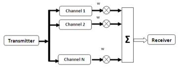
Figure 12: Equal Gain Combining
