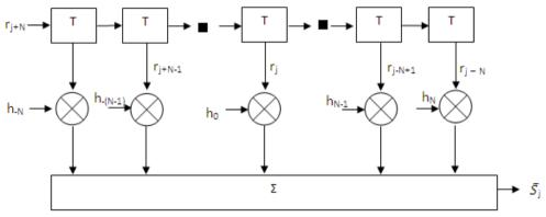
Figure 15: Transversal Filter equalizer (Schwartz, P49)
