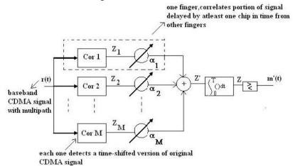
Figure 14 : A Rake Receiver
