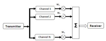
Figure 13: Maximal Ratio Combining
